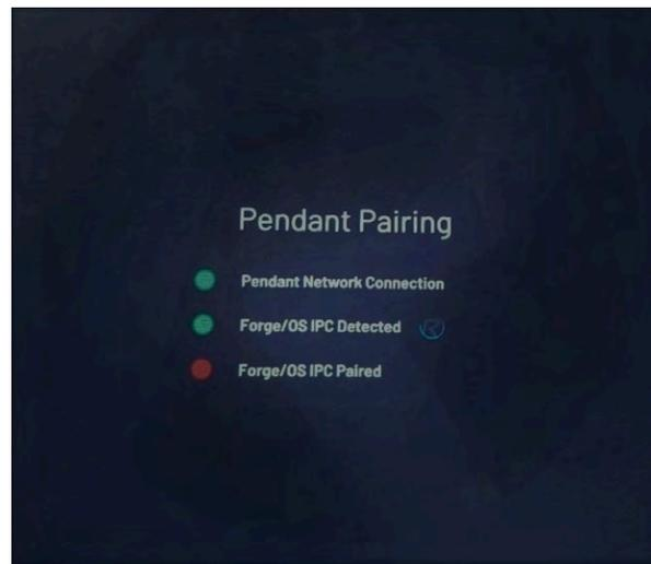
The UI shows the real-time state of each step. For example, if the pendant loses its network connection during pairing, all steps become undone.
